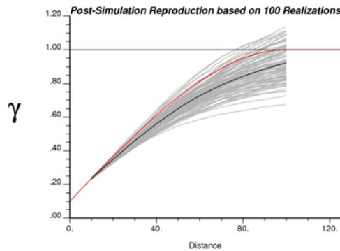
**Figure 2:** Post-simulation check for variogram reproduction based on 100 realizations. The red variogram shows the input model, the black line shows the average variogram of the simulated realizations, and the gray lines correspond to the variogram from each of the 100 realizations.
