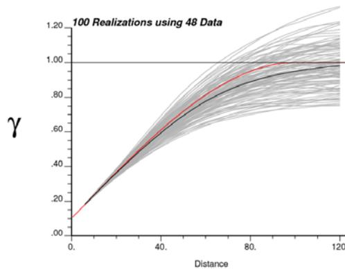
**Figure 3:** Post-simulation check for variogram reproduction based on 100 realizations using 48 data. The red variogram shows the input model, the black line shows the average variogram of the simulated realizations, and the gray lines correspond to the variogram from each of the 100 realizations.
