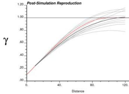
**Figure 1:** Post-simulation check for variogram reproduction based on 10 realizations. The red variogram shows the input model, the black line shows the average variogram of the simulated realizations, and the gray lines correspond to the variogram from each of the 10 realizations.
